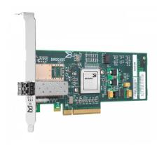
HPE 41B 4GB 1-PORT PCIE X4 FIBER CHANNEL HOST BUS ADAPTER, 571518-001
