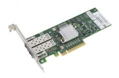
HPE 82B 8GB 2-PORT PCIE FIBER CHANNEL HOST BUS ADAPAPTER, 571521-01
